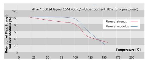
The flexural moduli and strengths of the Atlac® 580 resin over a temperature range of 20-180 °C were measured according to ISO-178. The laminates were based on 4 layers of 450 g/m² chopped strand mat with a fibre content of 30% w/w. Standard cure systems have been used and all specimen have been fully postcured.
